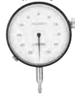
The high-precision type has a graduation of 0.5 µm.
